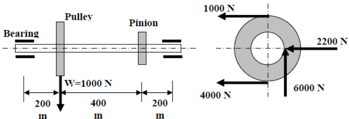
Q6. A shaft subjected to a torque of 4KN-m carries a bending moment of 1.5KN-m in vertical plane and 2KN-m in horizontal plane at a section. Determine its diameter and check for factor of safety. The determination of property in tension of the material of steel is quite reliable. The calculation of bending moment and torque is accurate. The shaft will be ground finished and heat treated to ultimate tensile strength of 700MPa with uniform micro structure.
