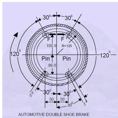
Q9. A spring set, hydraulically released double shoe drum brake, schematically shown at Fig 2 is to be designed to have a torque capacity of 600 N.m under almost continuous duty when the brake drum is rotating at 400 rpm in either direction. Assume that the brake lining is to be molded asbestos having a friction coefficient of 0.3 and permissible pressure of 0.8 MPa. The width of the brake shoe is to be third of drum diameter and the remaining proportion's are as shown in figure.
