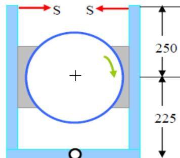
Q7. A differential band brake has brake drum of diameter 500mm and the maximum torque on the drum is 1000 N-m. The brake embraces  $\frac{2}{3}$ <sup>rd</sup> of the circumference. If the band brake is lined with asbestos fabric having a coefficient of friction 0.3, then design the steel band. The permissible stress is 70 MPa in tension. The bearing pressure for the brake lining should not exceed 0.2 MPa.
