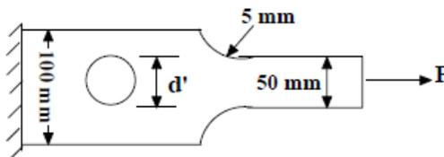
Q3. A rectangular stepped steel bar is shown in figure. The bar is loaded in bending. Determine the fatigue stress-concentration factor if ultimate stress of the materials is 689 MPa.
